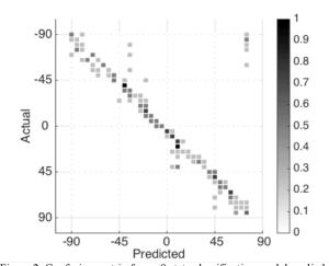
Figure 2. Confusion matrix for an 8 state classification model applied to a test data set.
