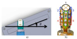
Figure 1. From [3], a) The arrow indicates the radial to ulnar motion of a right-handed index finger across a thick blade that is at an angle of  $\theta$  with respect to a body-fixed fingertip reference frame. b) The BioTac sensor electrodes were clustered into 6 regions of the fingertip.
